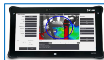
Figure 4 - Leak Quantification - QL320 Optical Gas Imaging System.
