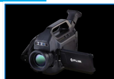
Figure 2-FLIR Camera to detect methane emissions.
