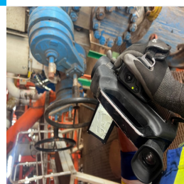
Figure 4 - Leak Quantification - QL320 Optical Gas Imaging System.
