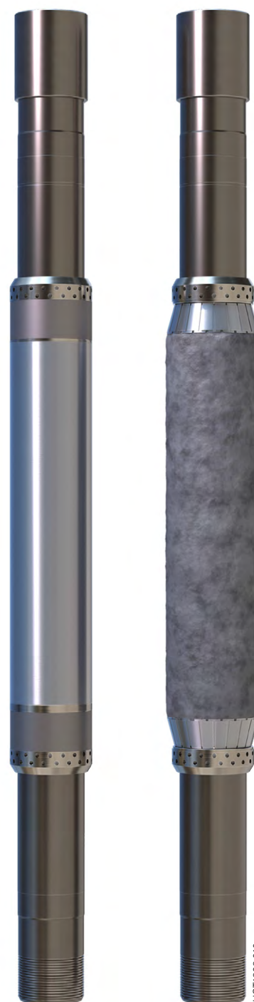
The Ovidius® expanding isolation system transforms from an engineered metal alloy into a rock-like material when it reacts with downhole fluids.
