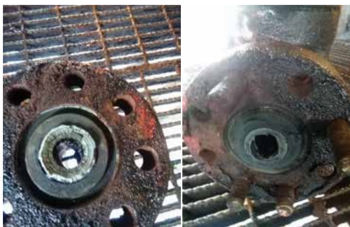
Annulus spool plugged with scale
