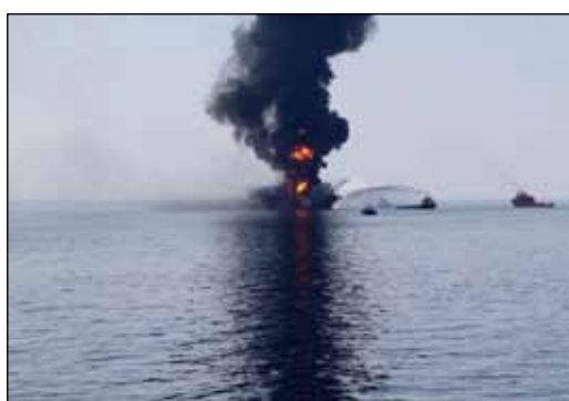
From top: support vessels using their fire fighting gear to cool the rig. About noon Day 1 – List is pronounced now
