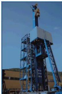
Figure 9. First offshore modular rack and pinion sidetrack drilling unit
