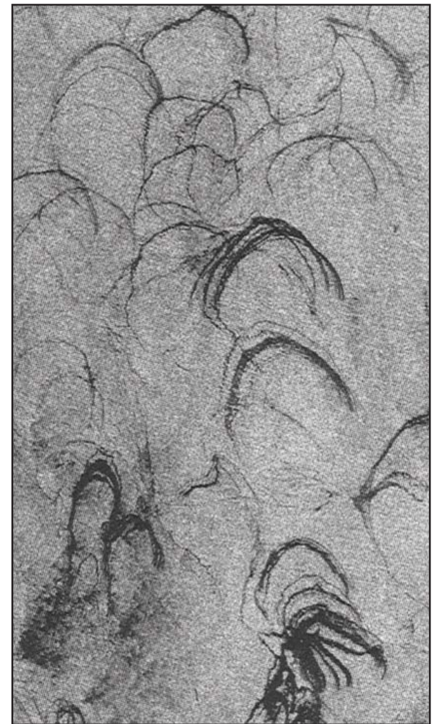
Natural oil slicks are detectable as black patches on this Radarsat ScanSAR Narrow subscene (100km x 100km) of Green Canyon, Gulf of Mexico acquired June 12, 1997. Wind variations associated with a frontal system are seen as two vertical dark lines in the center of the image.
