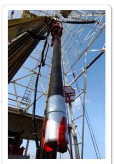
Weatherford's drilling-with-casing (DwC™) technique and Defyer™ DT series drillable casing bit, used with our  $\mathsf{Over}\mathsf{Drive}^{\scriptscriptstyle\mathsf{TM}}$  casing running and drilling system, successfully drilled casing 748 ft (228 m) TD in a single trip—reducing operator costs and eliminating nonproductive time in a challenging offshore environment.
